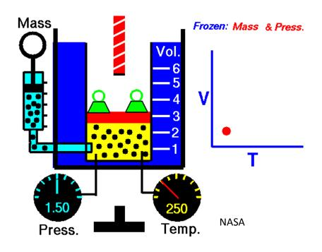
$$\frac{V_1}{T_1} = \frac{V_2}{T_2}$$
